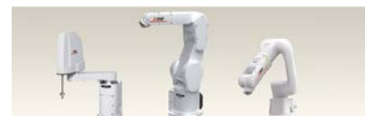
Robots: SCARA, articulated arm, cobots
